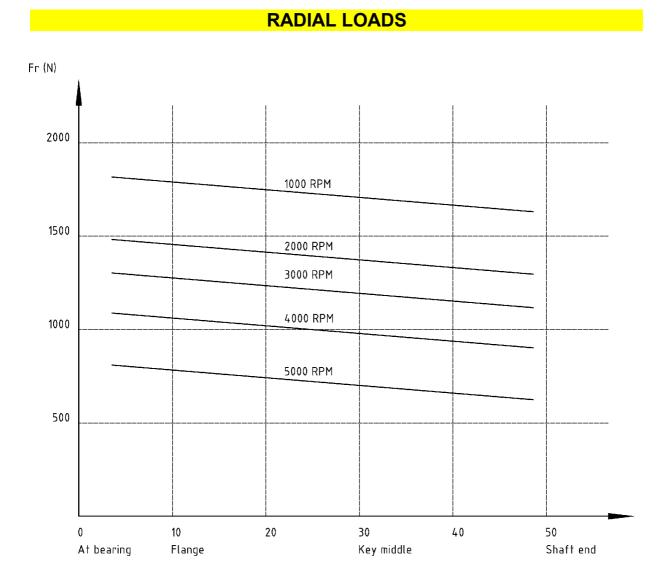
Maximal radial loads admissible on shaft, related to distance of application point (x) to flange and to speed, are given for a typical 20 000 hours bearing life.
